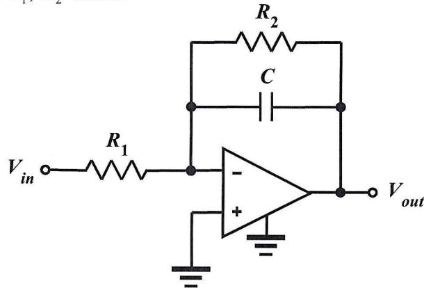
$$\frac{V_{in}}{R_1} + \frac{V_{out}}{R_2} + \frac{V_{out}}{\left(\frac{1}{j\omega C}\right)} = 0 \Rightarrow \frac{1}{R_1} V_{in} = -\left(\frac{1}{R_2} + j\omega C\right) V_{out}$$
